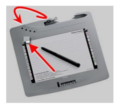
The Schoolpad connects to the PC wirelessly via Bluetooth communications. When the Schoolpad is powered on, it should automatically connect to the PC. You will hear 3-4 short beeps followed by a chirp indicating successful connection combined with the following message from the Interwrite Software in the bottom right hand corner of the screen.
