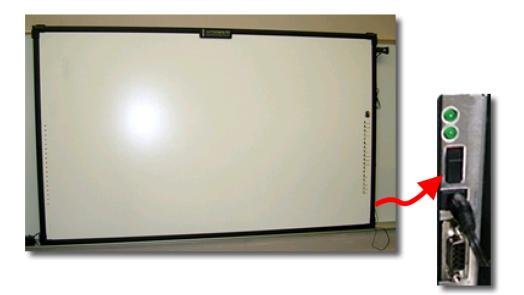
When the Schoolpad is powered on, it should automatically connect to the PC. You will hear 3-4 short beeps followed by a chirp indicating successful connection combined with the following message from the Interwrite Software in the bottom right hand corner of the screen. You can test the connection by moving the stylus over the pad; the mouse pointer on the PC should respond.
